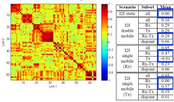
64 links – pairwise correlation subset – joint Rx, joint Tx, joint Rx or joint Tx, disjoint no link jointly High correlation if joint node is mobile
