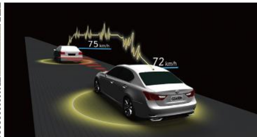
Communicating Radar Cruise Control (using vehicle-to-vehicle communication)
