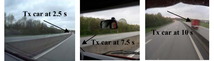
Fig. 5: General highway scenario and individual screenshots from the video of the measurement run: The Rx car passing by the Tx car and The Rx driving away from the Tx car (From LEFT to RIGHT)
