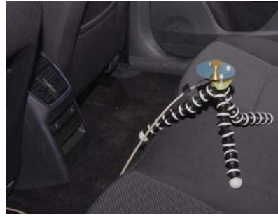
(b) 3–11 GHz monoconical antenna in the middle of the rear seat using a tripod.
