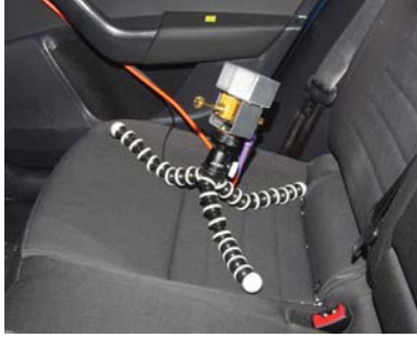
(c) The seat behind the front passenger with transmitting open ended waveguide antenna for 55–65 GHz. Please note the heat sink for the power amplifier cooling.
