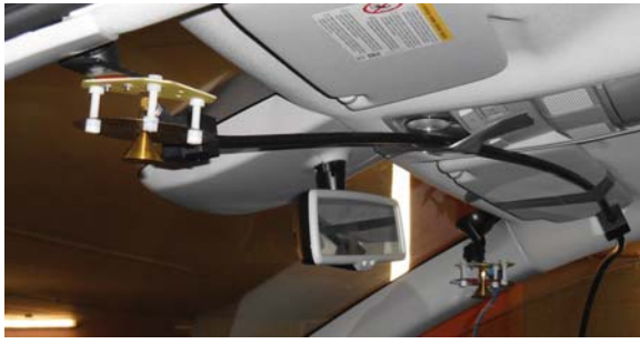
(a) 3–11 GHz monoconical antenna mounted on front windshield next to the rear-view mirror.
