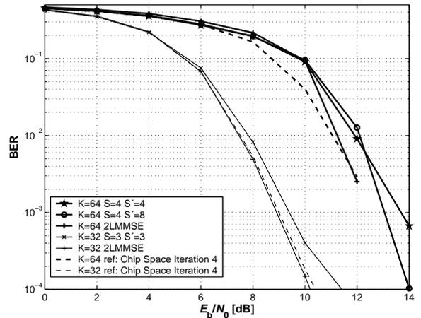
**Fig. 6. Krylov PIC in user space:** BER versus SNR after 6 iterations of the receiver. Channel estimation is using a Krylov subspace with dimension  $S \in \{3, 4\}$ , data detection is performed in user space with a Krylov subspace of dimension  $S' \in \{4, 8\}$  for  $K \in \{32, 64\}$  users. The dotted lines show the performances with PIC in chip space that we want to achieve.
