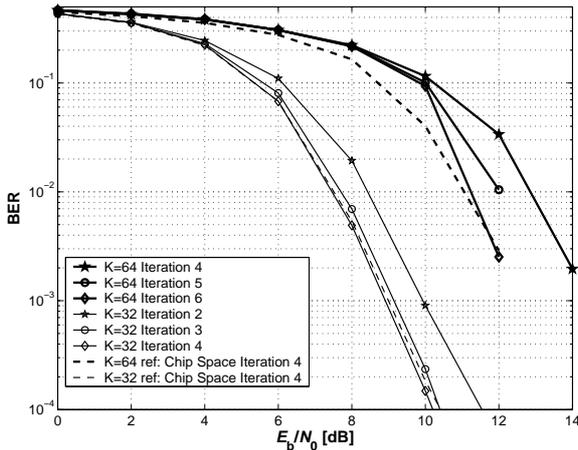
**Fig. 5. Iterative receiver performance with PIC in user space:** BER versus SNR after 4, 5 and 6 iterations of the receiver for  $K \in \{32, 64\}$  users. Both data detection and channel estimation are performed using the exact linear MMSE filter. The dotted lines show the performances with PIC in chip space that we want to achieve.
