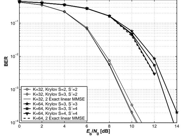
**Fig. 4. Krylov PIC in chip space:** BER versus SNR after 4 iterations of the receiver, time-variant channel estimation with a Krylov subspace of dimension  $S \in \{2, 3, 4\}$  and data detection with a Krylov subspace of dimension  $S' \in \{2, 3, 4\}$ , for  $K \in \{32, 64\}$  users.
