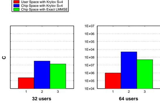
**Fig. 3. Computational Complexity for Data Detection:** for PIC in user space with Krylov approximated linear MMSE of dimension 4, PIC in chip space with Krylov approximated linear MMSE of dimension 4 and with exact linear MMSE, for  $K \in \{32, 64\}$  users.
