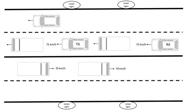
Fig. 4. Vehicular scenario: highway obstructed LOS
