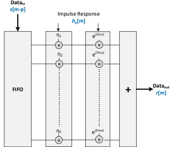
Fig. 2. Tapped-delay architecture
