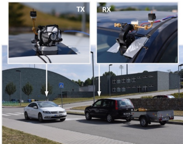
FIGURE 2. Measurement setup and environment of the opposite-lane passing V2V measurements at BUT.
