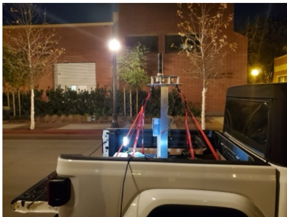
FIGURE 6. RX of the ReRoMA sounder loaded on the back of the pickup truck.
