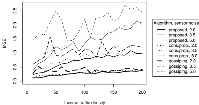
Fig. 5. Performance of the three algorithms for selected values of sensor noise.
