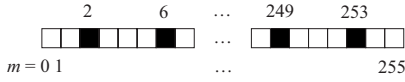
Fig. 2. Pilot pattern \mathcal{P} = \left\{ \left\lfloor i \frac{M}{J} + \frac{M}{2J} \right\rfloor \mid i \in \{0, \dots, J-1\} \right\} for block length M = 256 and J = 60 OFDM pilot symbols.
