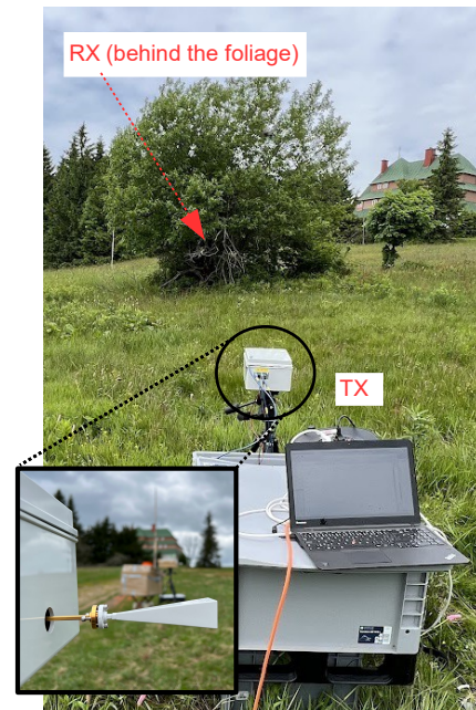
Fig. 1: Photograph of the 80 GHz channel sounder. The receiver (RX) is located behind the measured foliage. TX-RX separation is 30 m with the tree 15 m distant from the transmitter (TX).
